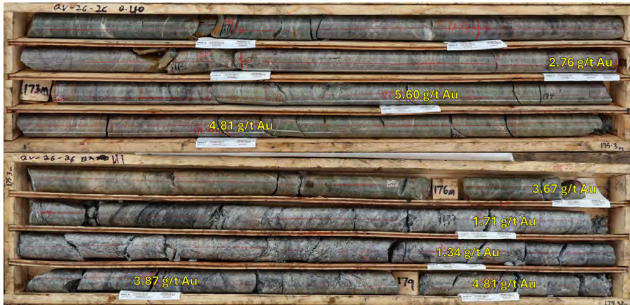
Figure 8 – Core photos hole QV26-026 with assays marked
